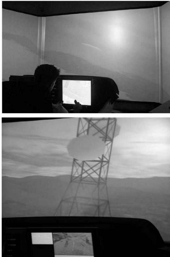
FIGURE 1 (a) Off-nominal outside-world traffic (the blimp is visible in the middle outside-world screen); (b) off-nominal radio tower.
