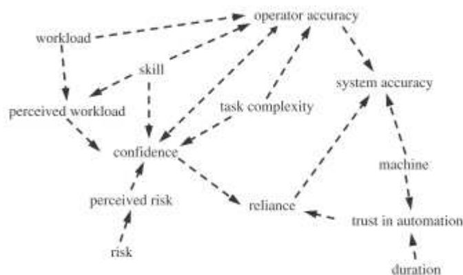
Fig. 1. Theory of operator reliance on automation (arrows indicate the hypothesized direction of influence) (from Riley, 1996, p. 21).
