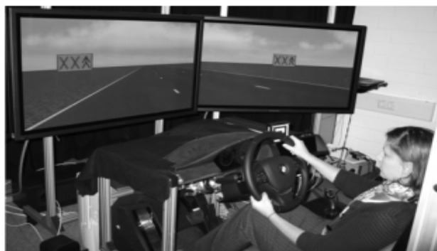
Fig. 2 Set-up of the ALCT with a car mock-up and plasma screens in a driving simulation environment
